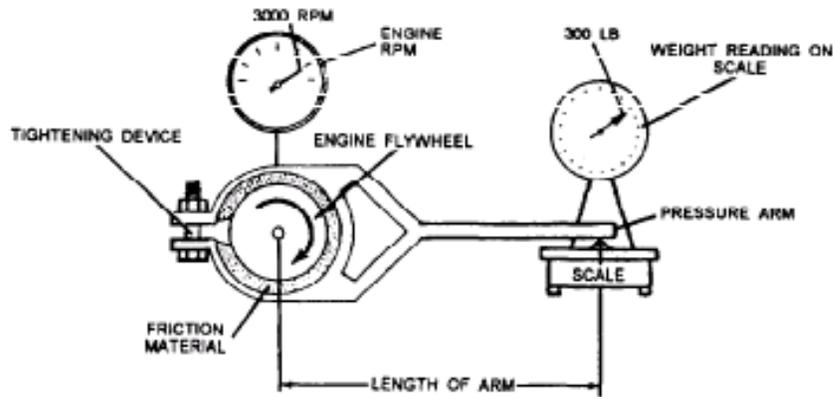
Figure 1. layout of a prony brake
