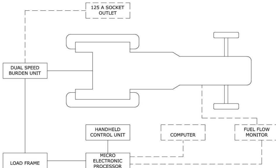
**Figure2. Schematic Layout of Froment Electronic Dynamometer**
