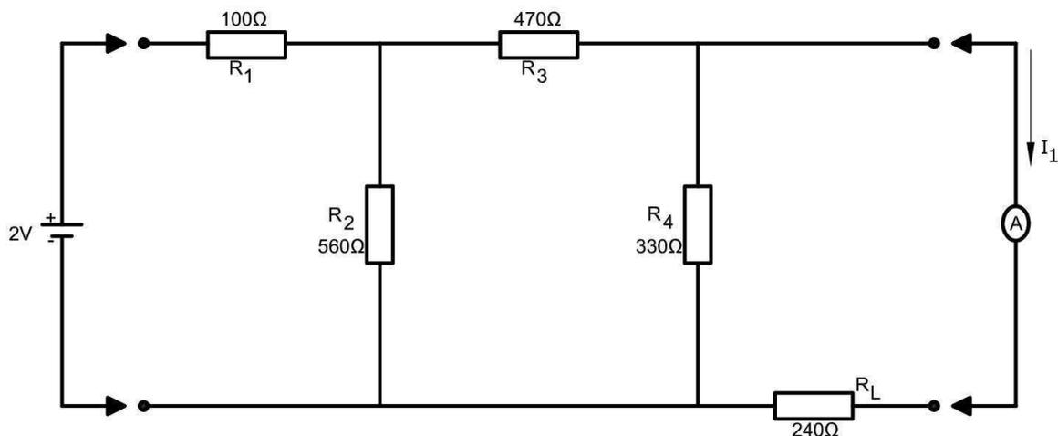
Find the current  $I_1$ , interchange the battery and ammeter and find, by calculation, the new current,  $I_2$ , through the ammeter. First find the currents,  $I_1$ , and  $I_2$ , as functions of  $V$ ,  $R_1$ ,  $R_2$ ,  $R_3$ ,  $R_4$  and  $R_L$ , then insert the values for the resistors. Make use of the results from question 1.
