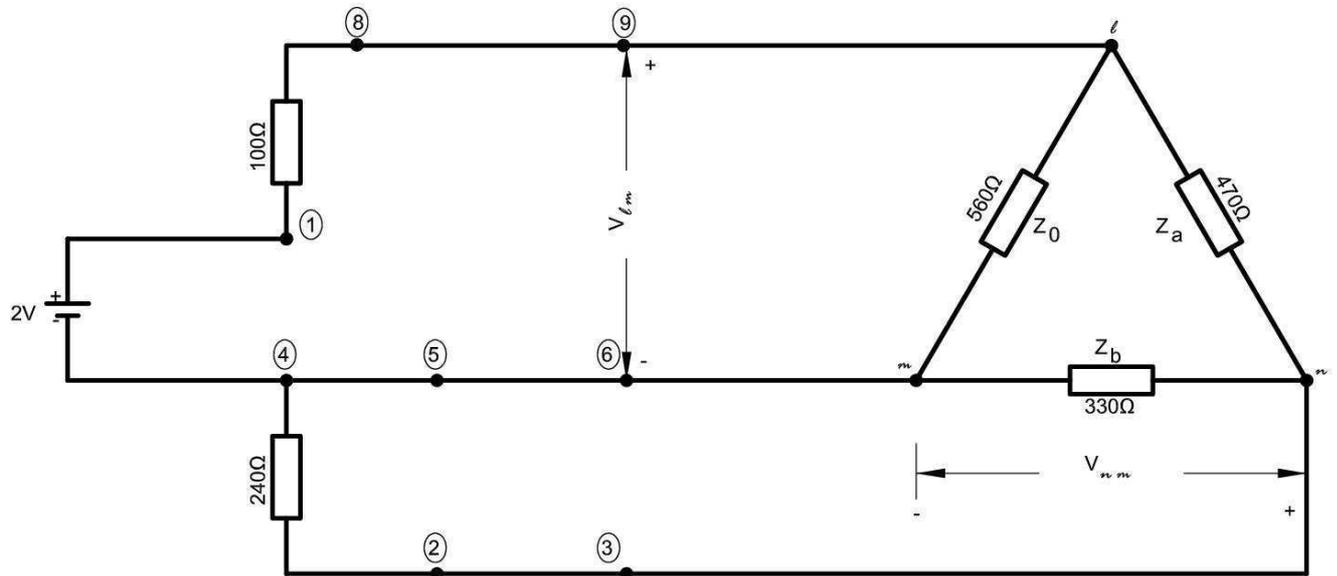
Links between 8 and 9, 5 and 6 and 2 and 3. Measure the voltages  $V_{lm}$  and  $V_{nm}$ .
