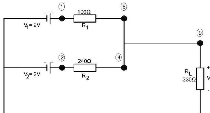
Point 4, 8 and 9 connect with links. Measure the voltage  $V$ .
