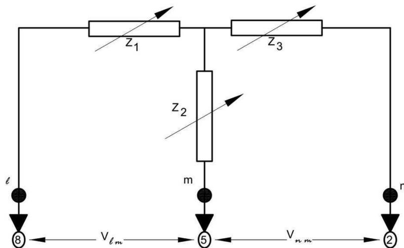
Measure the voltages  $V_{lm}$  and  $V_{nm}$ . How much do they differ from those found in 2 (a)?
