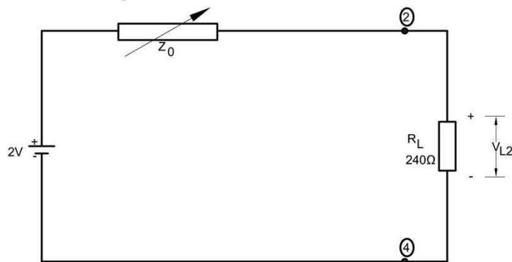
Set the variable resistor to  $Z_o$  and measure  $V_{L2}$ .
