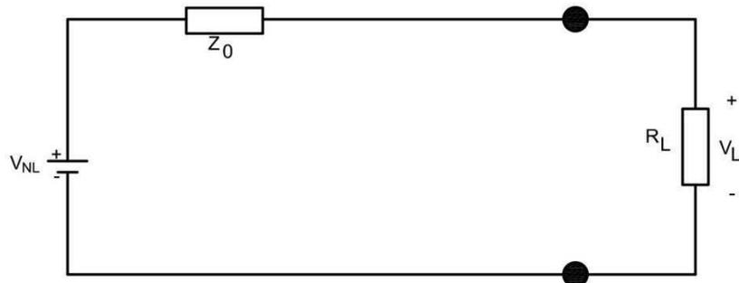
Find  $V_L$ ,  $V_{NL}$  and  $Z_0$  as functions of  $V$ ,  $R_1, R_2, R_3, R_4$  and  $R_L$  then insert the values.
