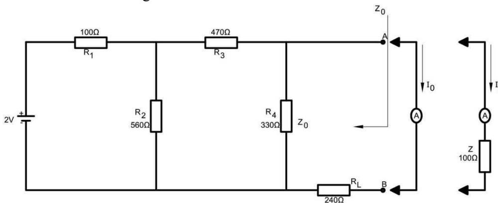
Find the output impedance  $Z_0$  between A and B. If an ammeter is connected between A and B find the current  $I_0$ .
