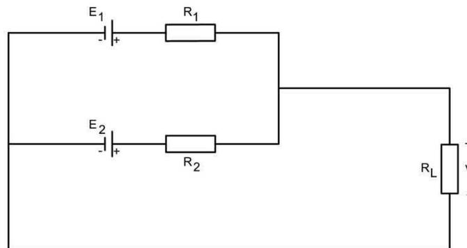
Fig. 2: Circuit of the Parallel Generator Theorem.
